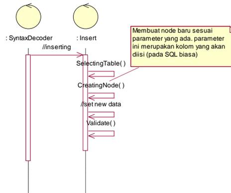
Gambar 16. Sequence diagram proses insert
