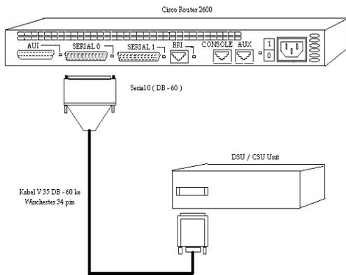
**Gambar 8 Koneksi Modem (DSU / CSU) ke Router**
