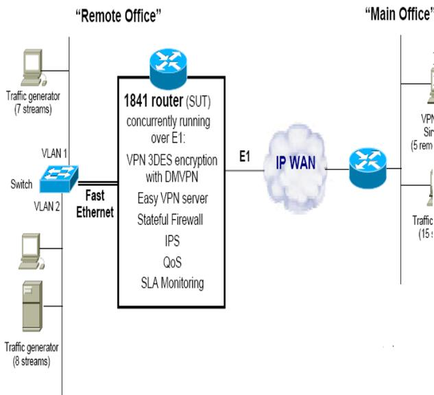
Gambar 12 Setup Uji Coba Router Cisco 1841
