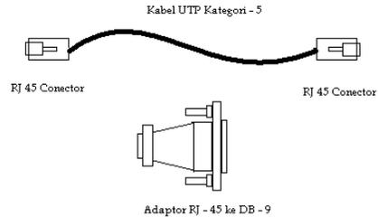
**Gambar 6 Kabel rollover & adaptor RJ-45 ke DB-9**
