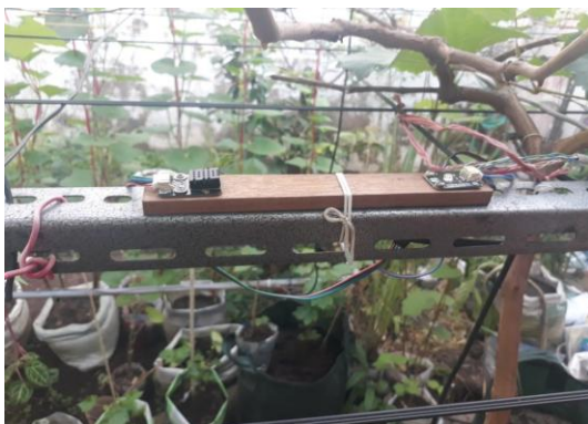
Fig. 3. Placement of temperature-humidity sensors and light sensors
