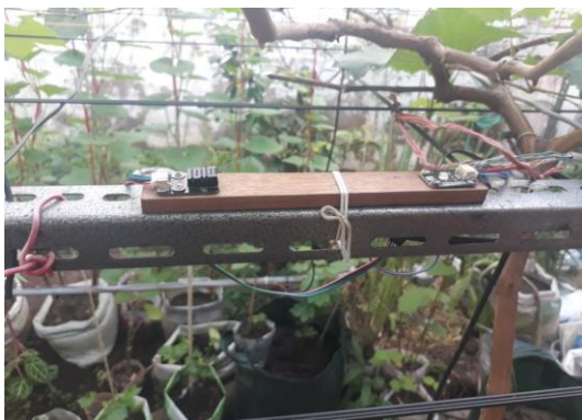
Fig. 3. Placement of temperature-humidity sensors and light sensors
